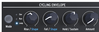
Der Cycling Envelope-Generator
